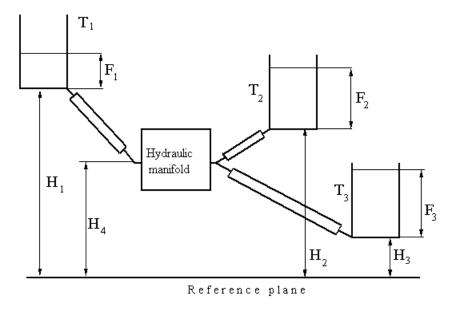
The models of tanks account for the fluid level heights F1, F2, and F3, respectively, and represent pressure at their bottoms as
