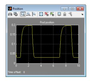
In the beginning, the valve is closed. Then, as the input signal reaches 50% of the actuator's nominal signal, the valve gradually opens to its maximum value and moves the cylinder rod in the positive direction. When the input signal goes below 50% of the nominal signal, the actuator closes the valve. The spring returns the cylinder rod to its initial position.
